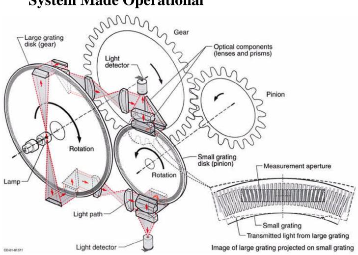
Schematic of the transmission error measurement system indicating the light path through the gratings and other optical components. At right is a representation of the light from one grating projected onto the other grating.
