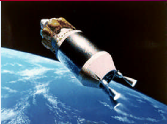
Expendable TLI Stage for First Lunar Outpost Mission using Clustered 25 klb, Engines -- "Fast Track Study" (1992)
