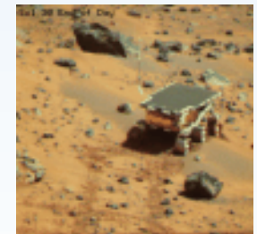
Photovoltaic Powered Mars Rover
