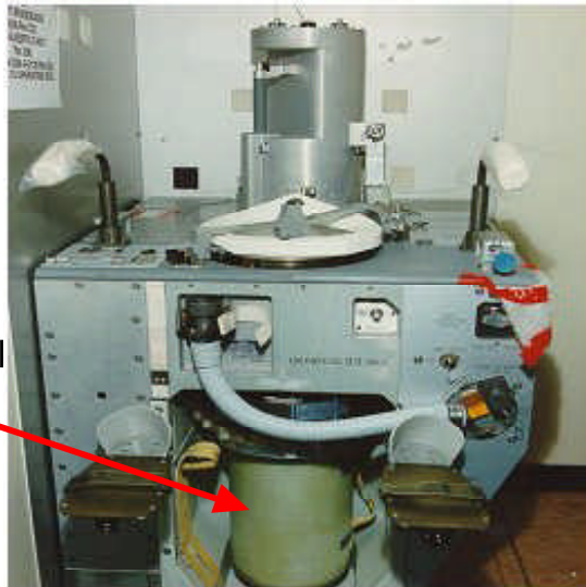
Waste Collection System
