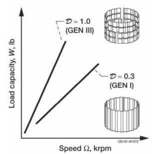
Foil bearing load capacity is enhanced by higher complexity in the elastic support (springs) structure.  $W = \mathcal{O}(L \times D)(D \times W)$ , where W is the maximum steady-state load that can be supported (N, lb),  $\mathcal{O}$  is the bearing load capacity coefficient (N/mm<sup>3</sup>-krpm, lb/in.<sup>3</sup>krpm), L is the bearing axial length (mm, in.), D is the shaft diameter (mm, in.), and W is the shaft speed in 1000 rpm (krpm).
