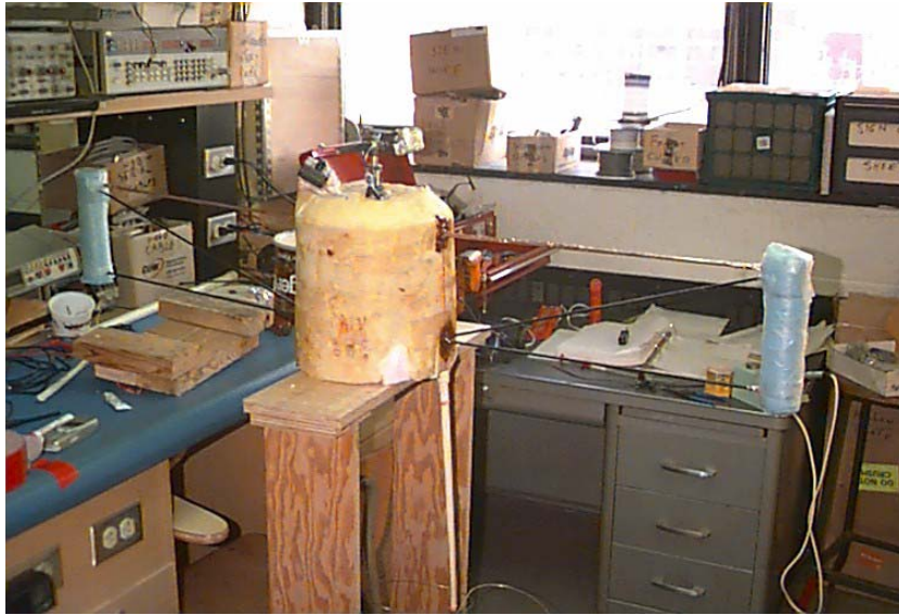
Figure 3. Suntracker scientific package developed for characterizing multi-junction solar cells in the stratosphere.
