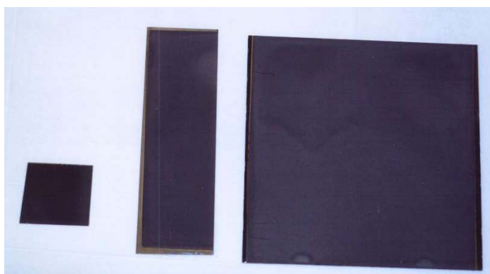
Figure 16. Increase in substrate sizes from 1.25" x 1" to 1" x 4" to 4" x 4"
