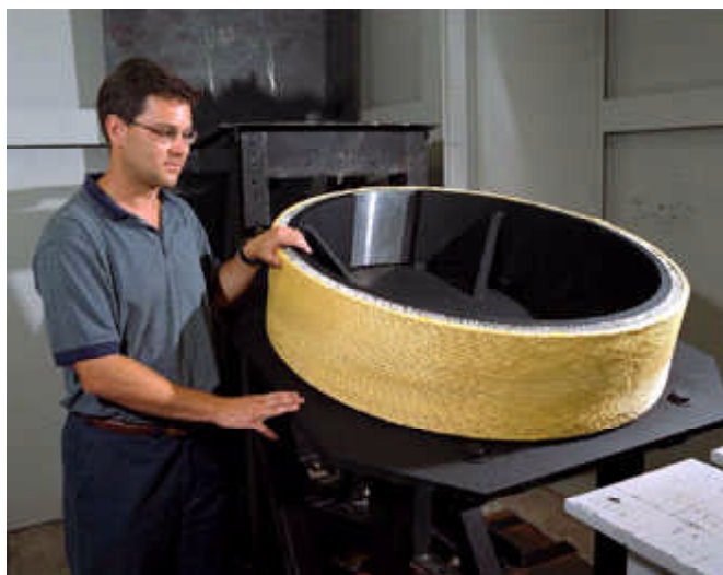
Test specimen mounted on a fixture in front of the impact gun. The specimen is supported at a slight incline so that the projectile can impact it from the inside.
