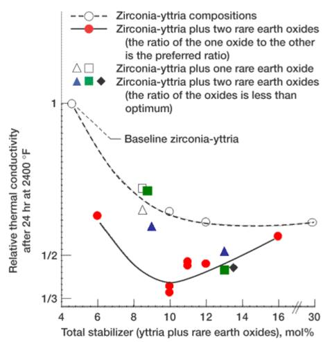
Thermal conductivity, k, after 20 hr of exposure in the laser rig test. The plot shows an approximately 40-percent reduction in the thermal conductivity of the preferred compositions, which are represented by the solid circles.
