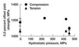
Tension (triangles) and compression (circles) yield strength as a function of hydrostatic pressure.
