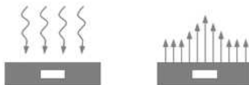
Flash thermography setup. Left: A specimen is heated with a pulse of thermal energy. Right: As the thermal front conducts through the material, defects such as delaminations prevent the flow of heat and result in a higher surface temperature directly above the specimen.
