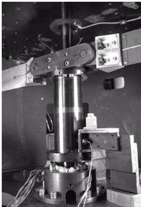
A two-bladed rotor, oriented vertically, which is supported by a radial active magnetic bearing used for active blade vibration control in the NASA Glenn Dynamic Spin Rig facility.
