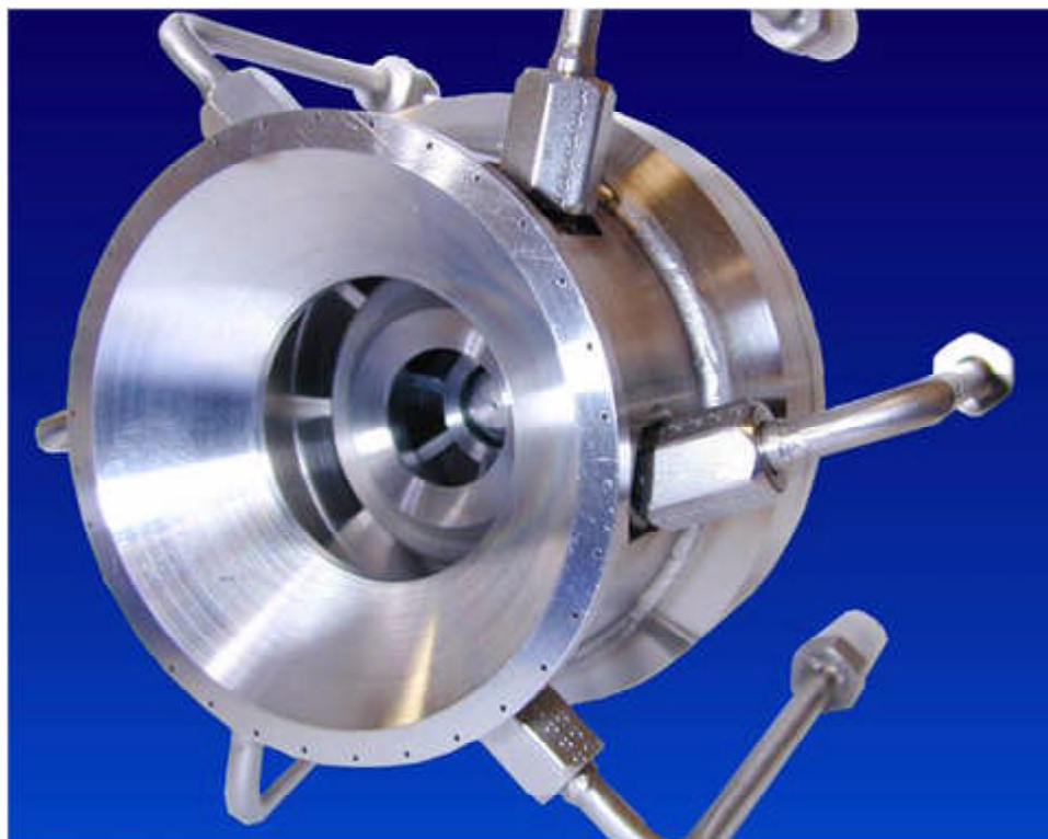
Ultra-low-NO x combustor concept that injects fuel from the wall of a venturi section (LDWI), counter to the air swirl. The air swirl is generated upstream of the Venturi section. Shown is a module for flame-tube testing with an enclosed pilot burner.
