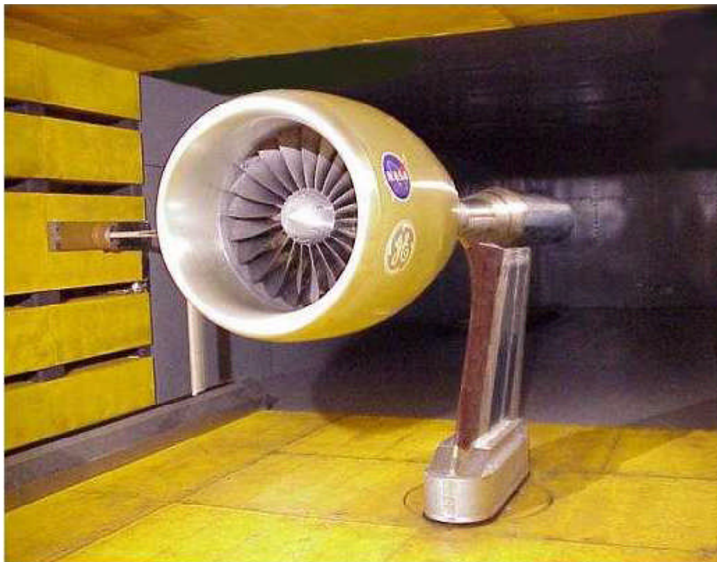
The 22-in. rig used for the Fan Noise Source Diagnostic Test shown in Glenn's 9- by 15-Foot Low-Speed Wind Tunnel.
