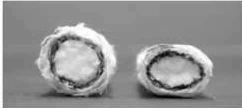
Seals before (left) and after (right) 1900 °F temperature exposure.
