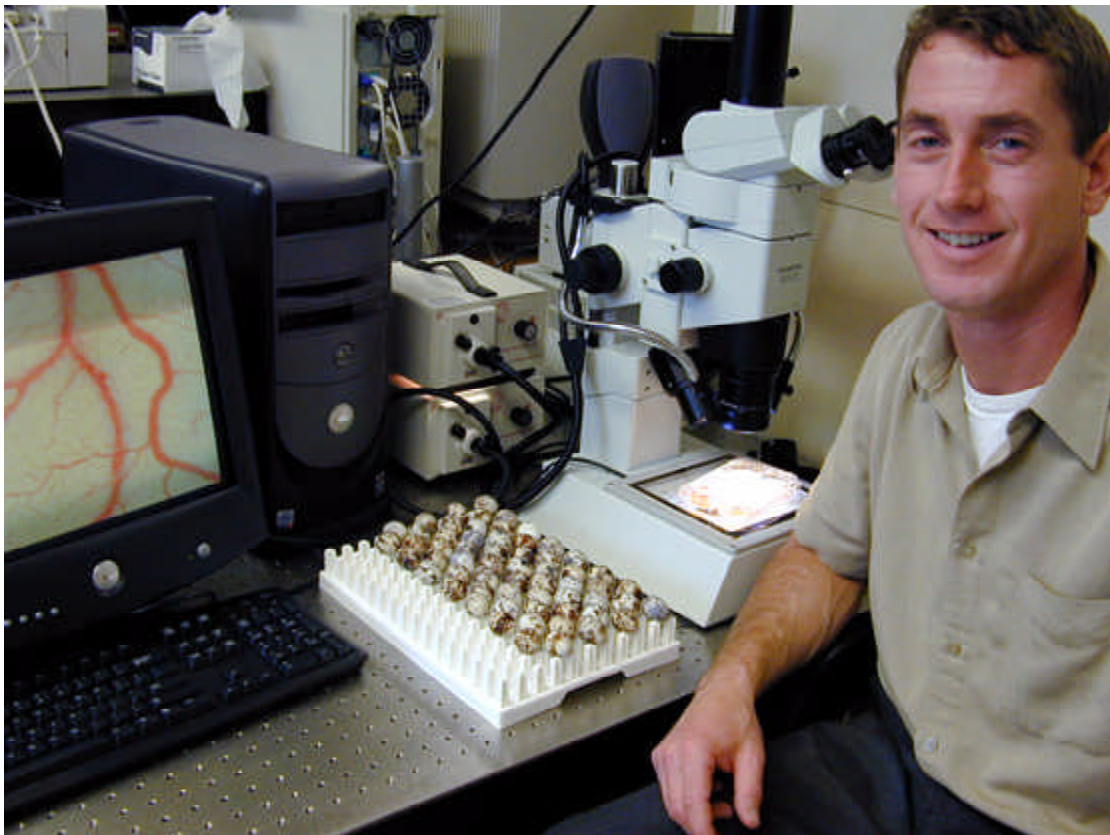
Mike Bronczek is imaging blood vessels in quail eggs intravitaly prior to fractal-based quantification of blood vessel growth after culturing the eggs (shown on the white tray) in the new Vertebrate Cell Culture Facility at Glenn.
