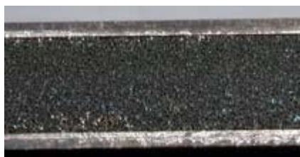
Side view of a 17-4 stainless steel foam panel with face sheets.
