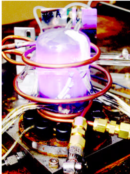
IN 718 heater head at 650 °C (1200 °F) with an induction heater coil.
