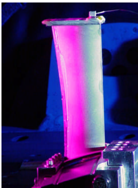
Coated stator vane on the shaker slip table. Total vane height is approximately 15 cm (6 in.).
