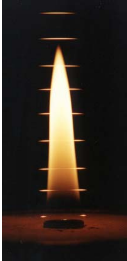
Image of the test flame and glowing fibers. The flame is about 70 mm long. The flame was observed in normal gravity with the flame tip up.
