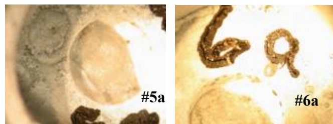
Figure 5: Iron oxides processed in \text{CO}_2 (#5a) \text{Fe}_3\text{O}_4 , (#6a) \text{Fe}_2\text{O}_3
