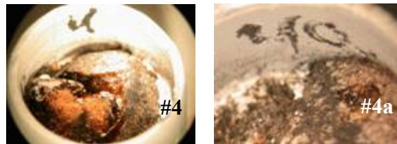
Figure 9: Simulant disks with 10% carbon added (#4) has a strongly magnetic chunk, (#4a) not as strongly magnetic
