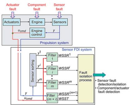
Architecture of the sensor fault detection and isolation (FDI) system, where u<sub>cmd</sub>, control commands; y, sensor measurements; y<sup>i</sup>, subset of sensor measurements used by filter i; WSSR (weighted sum of squared residuals), fault indicator signal; WSSR<sup>i</sup>, fault indicator signal generated by filter i; WSST, fault indicator signal (weighted sum of squared tuners).
