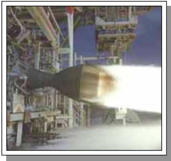
Figure 2, MC-1 (Fastrac) thrust chamber assembly being tested at MSFC
