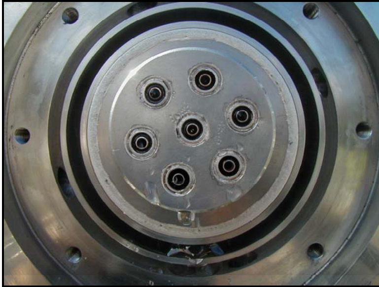
Figure 23. LO 2 /LH 2 Multi-Element Injector.
