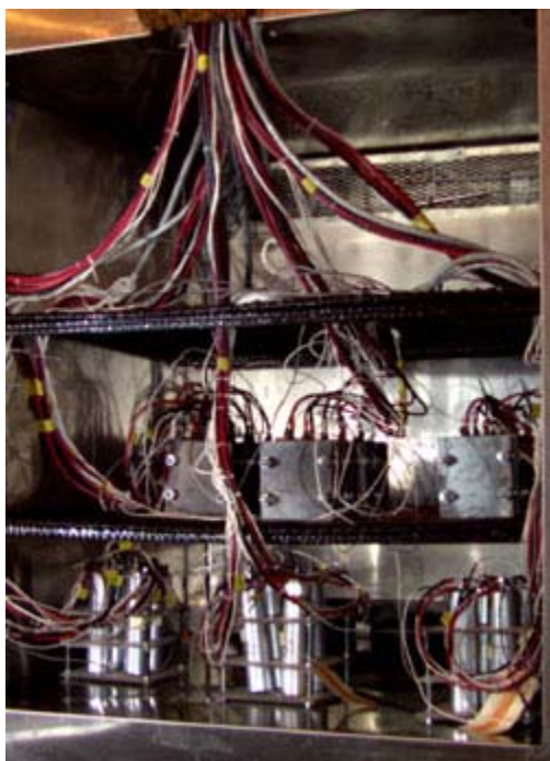
Lithium-ion cells from Saft and Lithion installed in a test chamber.
