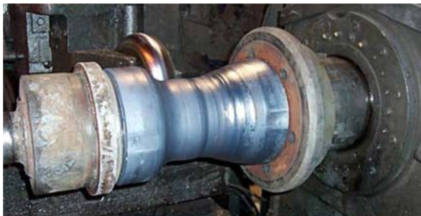
Metal spinning of GRCop-84 into the final hourglass-shaped liner preform.
