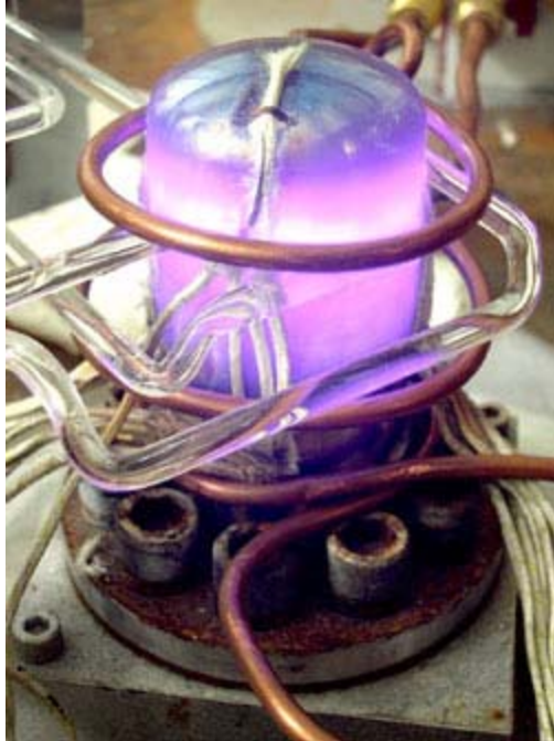
Three-month test of IN 718 heater head at 650 °C (1200 °F) with induction heater coils and diametral extensometer quartz glass probes.
