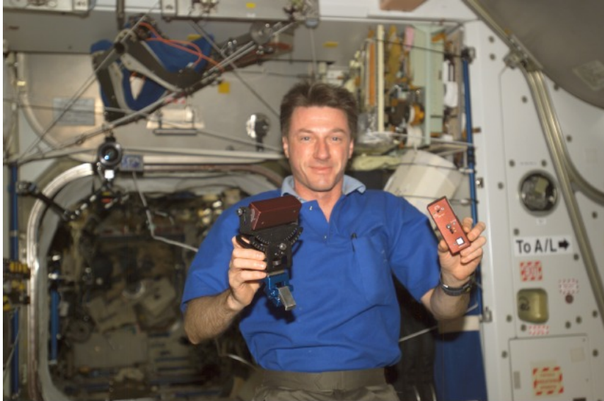
Expedition 8 Commander Michael Foale holds the SPHERES ultrasound beacon and beacon tester while performing functionality checks between the beacon/beacon tester and its proximity to a general luminaire assembly in Unity Node 1.
