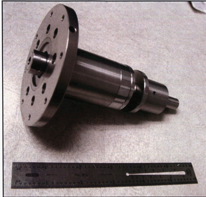
Figure 7. Custom Differential Satellite Roller Screw
