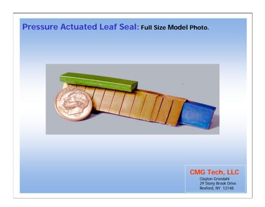
Leaf seal radial height and axial length is small, of the order of 0.5 inches as shown.
