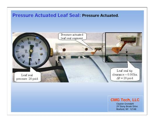
Pressurized model shows small clearance under leaf tip with differential seal pressure applied.
