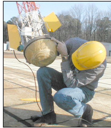
Fig. 8. Impact Absorber, Post-Test
