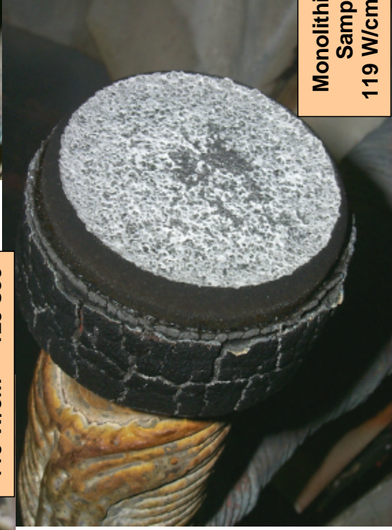
Strip-Collar Bonding Sample 3085 119 W/cm 2 – 125 sec
