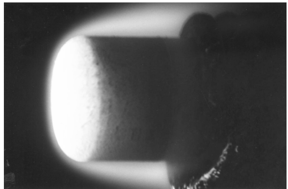
Fig. 6. AQ60 sample during IRS plasma test
