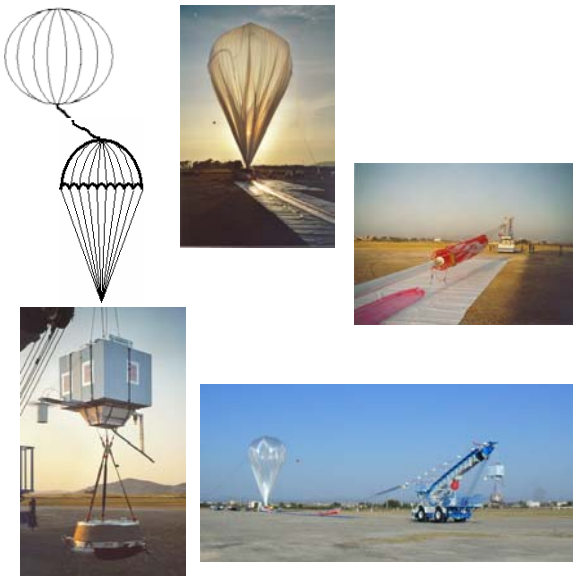
Fig. 6 The flight train: balloon, parachute, ASI telemetry gondola and Huygens mock-up with onboard HASI.
