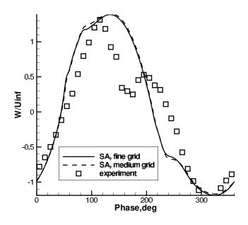
Figure 2: Vertical velocity component at the orifice exit.
