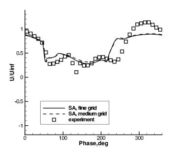
Figure 3: Streamwise velocity component at the orifice exit.
