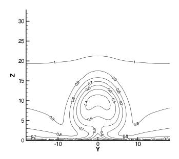
Figure 5: Contours of  $U/U_{\infty}$  at x=76.2 mm (4D downstream), phase=200°, SA on medium grid.
