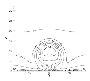
Figure 4: Contours of  $U/U_{\infty}$  at x=76.2 mm (4D downstream), phase=200°, SA on fine grid.
