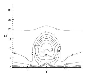
Figure 6: Contours of  $U/U_{\infty}$  at x=76.2 mm (4D downstream), phase= $200^{\circ}$ , SST on medium grid.
