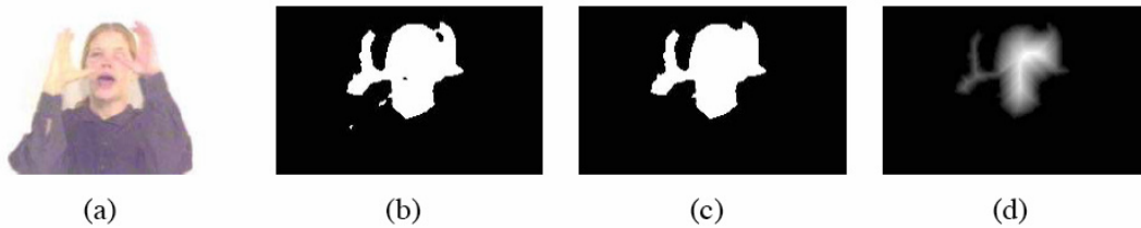
Figure 4. Preparation of the skin color mask for the EM algorithm. (a) Original image, (b) Threshold segmented skin color probability, (c) Skin color mask with holes removed, (d) Distance transformed skin color mask.
