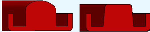
Cross-sections of the elastomer seal concepts with elliptical top (left) and flat top (right) sealing surfaces.
