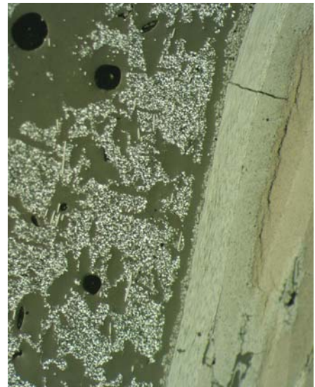
Optical images of GRC 2 at 50 X. The picture (right) shows the interaction of GRABER and the SiC coating. To the left is an image of the gasket material after heating.
