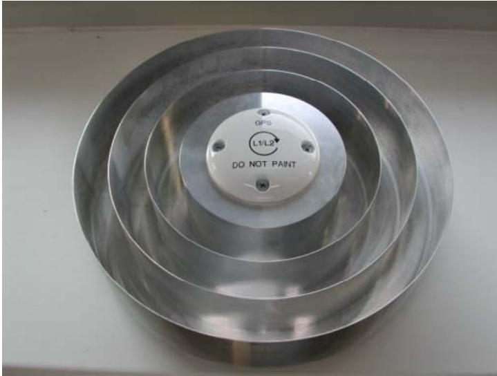
Fig. 9 GPS antenna and choke ring for the TSX/TDX satellites (engineering model).
