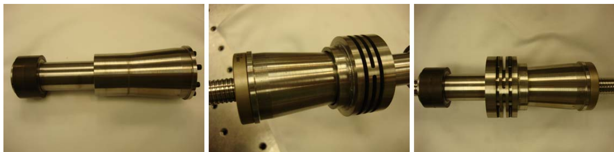
Figure 6: Bearing Preload Flexure and Rotor mounted to Drive Link
