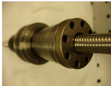
Figure 9: Ballnut bolted to Drive Link
