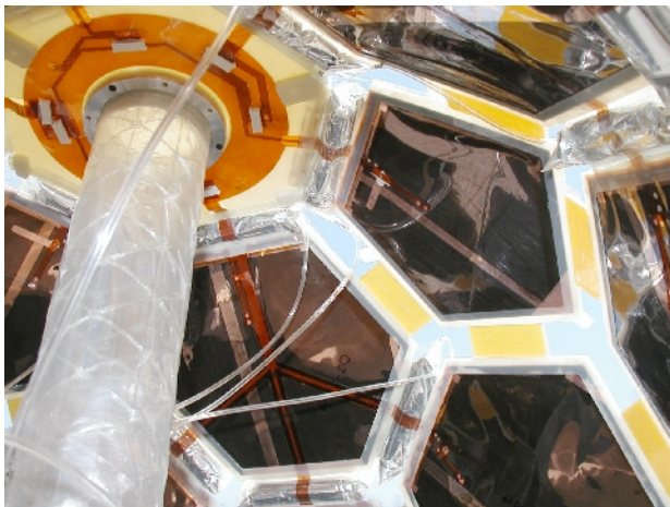
Figure 12. Interior of Hemisphere while Being Cured in Sunlight
