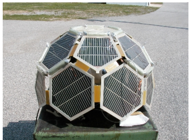
Figure 13. Curing of the EDU Hemisphere in Sunlight
