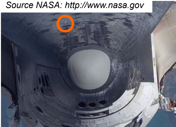
Figure: heat shield of the Space Shuttle in orbit during flight STS-114 with gap filler sticking out.
