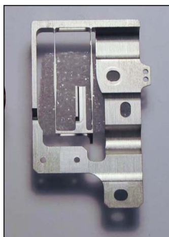
Figure 4: Micro-milled and passivated shutter structure.
