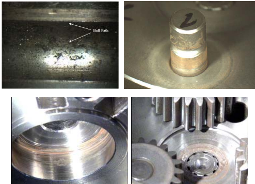
Figure 3: Lubrication failure of first actuator after life test 1
