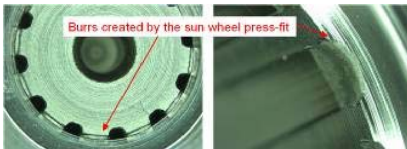
Figure 16: Failed pressing trial results
