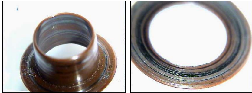
Figure 12: Pre-QM1 Vespel SP1 Bushing and Distance Washer after life test
