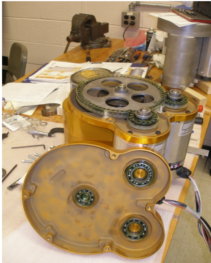
Figure 11. New Gearbox, Lid Removed
