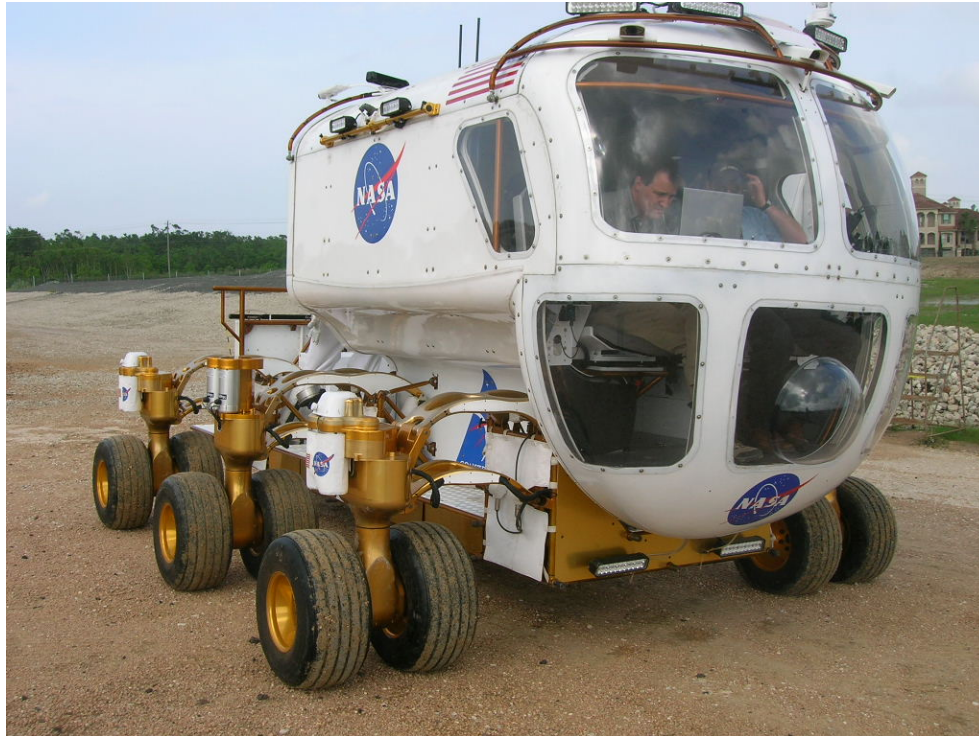
Figure 3. LER Starboard Center Wheel Pod with New Gearbox
