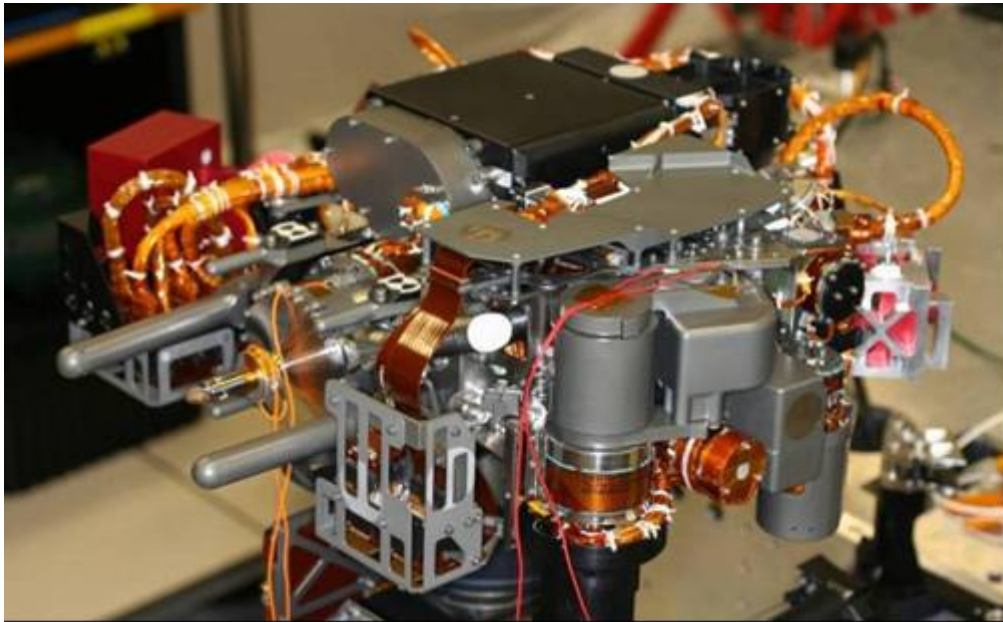
Figure 10. The assembled EM Turret with the Drill, CHIMRA, and Instrument Isolators installed. Mass models are used for the DRT, APXS, and MAHLI.
