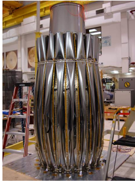
Figure 1: Stowed TacSat-4 UHF Antenna
