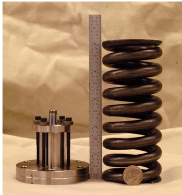
Figure 3. Piston/Cylinder Actuator (Left), And Spring It Compressed (Right) During Actuation
