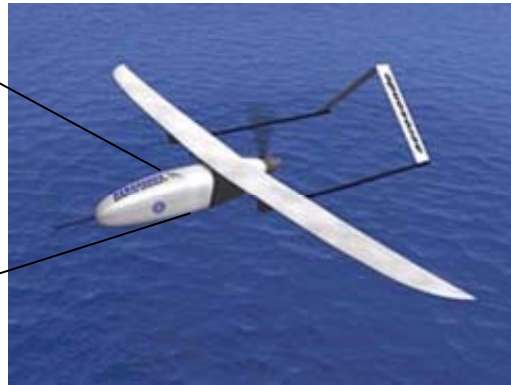
Figure 22. Modular Radiometer on board UAV
