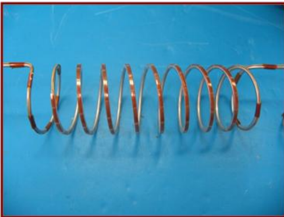
Figure 4. Outer Propellant Tubing with Heater
