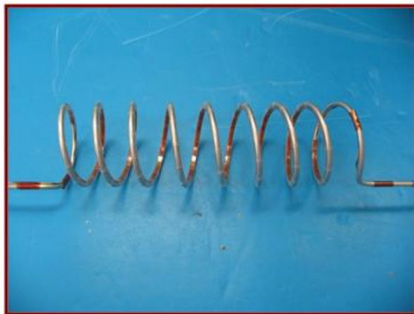
Figure 5. Inner Propellant Tubing with Heater
