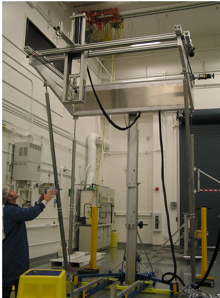
Figure 13: Pair of triangulated roll poles to stiffen telescoping tower of industrial lift
